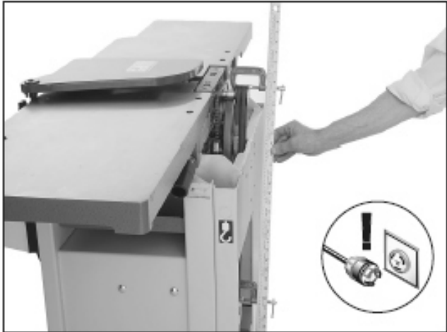
Figure 47. Checking belt alignment.
